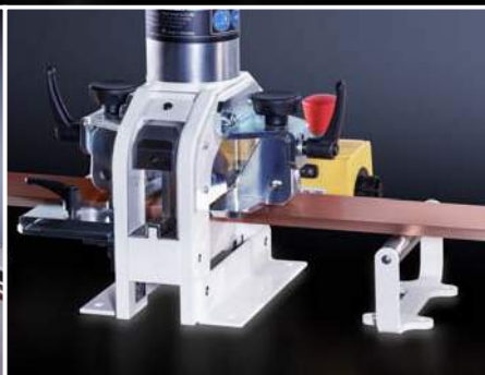
Cutting a busbar to length
