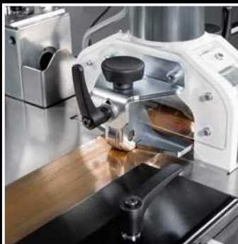
Cutting busbars to length with integral precision laser
