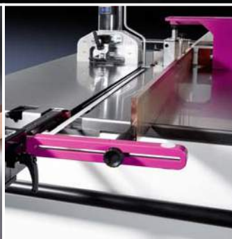
Punching busbars, pull-out measurement system
